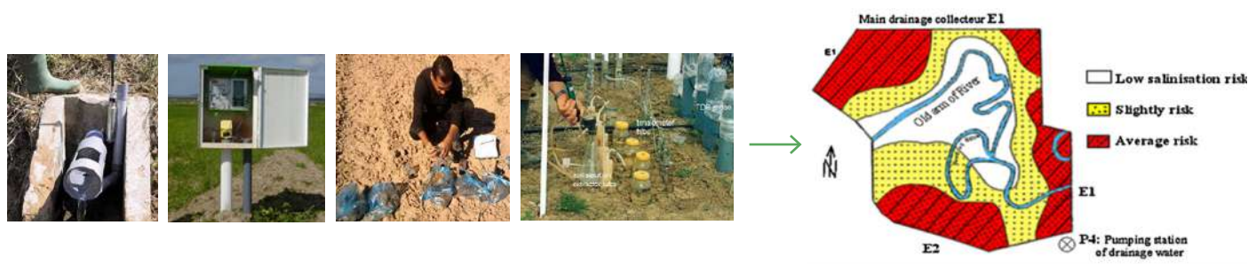
Figure 1. Monitoring of water (surface water table, drainage, irrigation) and soil properties for the zoning of units with different degrees of risk of soil salinization in the irrigated perimeter of Kalaat al Andalous (Bouksila et al., 2013).
