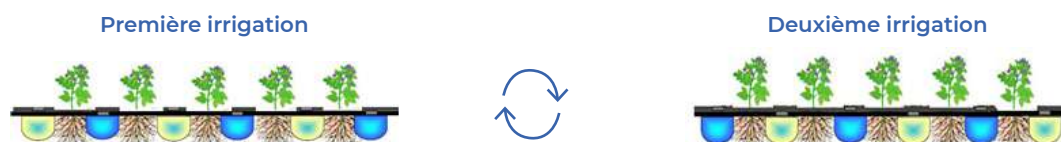
Figure 1. Experimental setup of an irrigation system by partial drying of the roots of potato.
